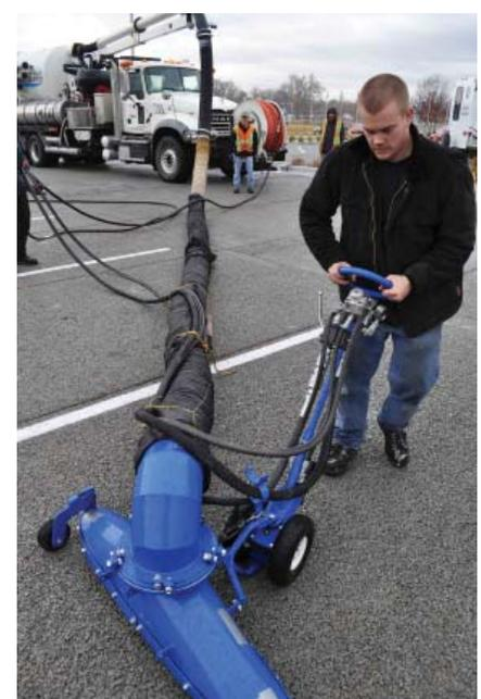
Vacuum pumps fall into two categories, positive displacement type and fan type. Performance is measured in pressure and volume. The BIRD Vacuum needs at least 3,000 cfm of air volume to operate effectively and the negative pressure starts at around 7 inches of mercury (Hg). Another expression of vacuum pressure is stated as feet of water.
