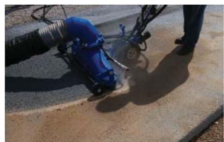
Positive displacement type vacuum trucks will typically displace 3,000 to 6,000 cfm of air at significantly greater pressure. For vacuum units with sufficient horsepower and positive displacement, you can expect up to 27 in.Hg. This configuration brings the BIRD Vacuum to high performance. This is not an economy mode of operation but is certainly effective in restoring permeability.
